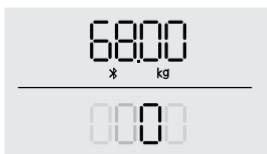
If the number flashes twice, that means the weight measurement is complete. When the number 0 stops moving across the screen from left to right, that means the body analysis is complete.
