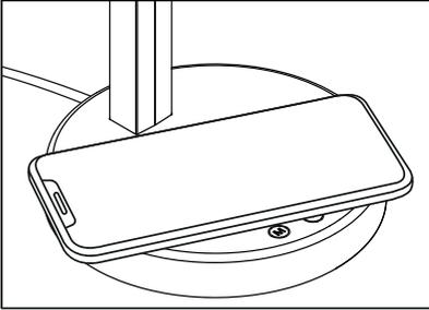
Your Qi-compatible phone can be charged by placing it on the **Wireless Charging Area** on the lamp base. To charge wirelessly, place your device on top of the charging icon at the center of the base. The device must be placed directly over the icon for the charging function to work optimally. Note that it may be necessary to activate wireless charging in your device settings.
